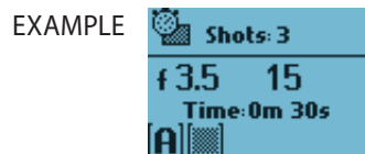
Screen after Interval setting activated indicating 3 shots remaining at 30 second intervals.
