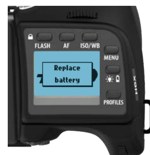
Exhausted battery warning
