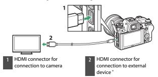
\* Choose a cable with a connector that matches the connector on the HDMI device.
