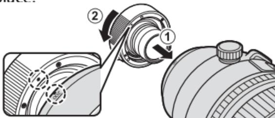
**3** Align the camera mounting index on the teleconverter with the index on the camera (①) and rotate the lens and teleconverter assembly in the direction shown (②) until it clicks into place.
