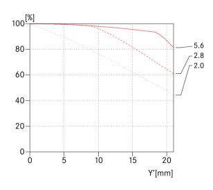
Distortion is the deviation of the real image height (in the picture) from the ideal image height. The relative distortion is the percentage deviation. The ideal image height results from the object height and the magnification. The image height of 21.6mm is the radial distance between the edge and the middle of the image field for the format 24mm x 36mm. The graph of the effective distortion illustrates the appearance of straight horizontal and vertical lines in the picture.
