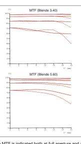
The MTF is indicated both at full aperture and at  $\ensuremath{\text{f/5.6}}$  at long taking distances (infinity). Shown is the contrast in percentage for 5, 10, 20 and 40 lp/mm accross the height of the 35 mm film format, for tangential (dotted line) and sagittal (solid line) structures, in white light. The 5 and 10 lp/mm will give an indication regarding the contrast ratio for large object structures.The 20 and 40 lp/mm records the resolution of fine and finest object structures.
