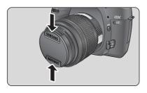
Take off the lens cap by pressing the two tabs inward as shown above.
