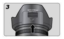
3. Attach the PL filter window cap.
