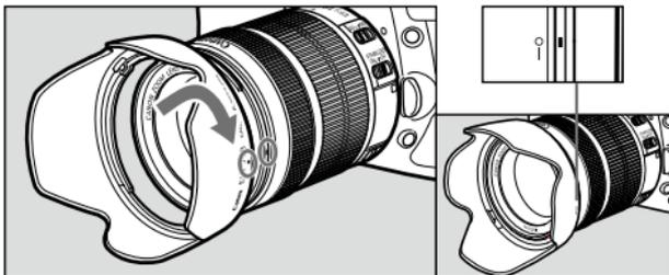
The EW-73B hood cuts out unwanted light and protects the front of the lens from rain, snow, and dust.
