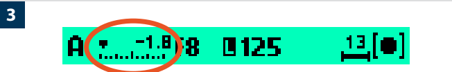
New metered area is 1.8 EV lower than the area metered when the AE-L button was pressed.
