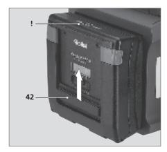
**42** up. This will open the drawslide, lock the magazine on the camera and release the shutter button.
