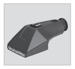
The 90° **High-Eyepoint View-finder** gives an upright, right-side-up view-finder image magnified 3.4x. Its eyepiece can be easily adjusted from +4 to -4 diopters. Its display is automatically switched to laterally correct presentation. The High-Eyepoint View-finder can likewise be used in four different positions spaced 90° apart.
