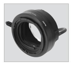
The **reversing adapter** further extends the camera's versatility in close-up photography. It allows reverse-mounting of any lens with a size VI filter bayonet. The camera's exposure and exposure-metering modes remain fully functional. It is advisable to combine use of the reversing adapter with that of a bellows attachment. With a reverse-mounted 80mm f/2.8 Xenotar, for example, available magnifications range from 1.8x to 3.5x.
