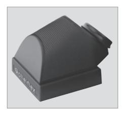
The 45° **Prism-finder** gives an upright, right-side-up view-finder image magnified 2.5x and can be used in four different positions spaced 90° apart so that it makes for comfortable viewing even in awkward shooting positions. As the viewfinder is mounted, its display is automatically adjusted for laterally correct presentation.
