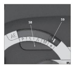
Set exposure-mode selector **59** to red index, switch camera on with master switch **60** and briefly depress the shutter release to stage 1. Viewfinder and handgrip displays are activated.
