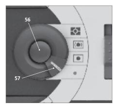
Set metering-pattern selector *57* to the red index. If necessary, switch camera on with master switch *60* and briefly press the shutter release to stage 1. This will activate the view-finder and handgrip displays. Keeping menu button *58* depressed, you can correct selected EV values by turning shutter-speed dial *25* and vary ISO values from ISO 12 – 3200 with the aid of aperture dial *21*.
