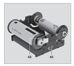
Make sure that the paper leader moves over the pressure plate to the empty spool *44* according to the symbol *45*.
