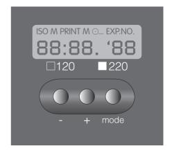
As the batteries are loaded, all segments of the LC display should light up simultaneously for about one second. Should this check fail to appear, briefly push battery spring *a* away from the batteries and let go.
