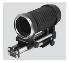
The **bellows attachment** features a precision rack and pinion and a focusing stage. Clamps serve to lock the extension between 67 and 204 mm. The latter can be read off a scale. A 1/4" tripod socket is provided. All exposure and exposure-metering modes of the camera remain fully functional when used in conjunction with the bellows attachment.
