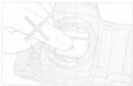
1. Blow lens with blower or blower screen. Remove dust with a blower brush.
