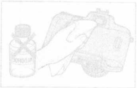
7. Clean viewfinder eyepiece and LCD panel with a soft, clean cloth. Do not use liquid cleaners.
