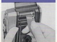
The NIKKOREX F accepts any standard 35 mm black-and-white or color film of 20 or 36 exposure load. Loading should not be made in direct sunlight, but in subdued light.
