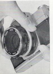
To remove the lens, hold the camera as shown left, depress the lock button found underneath the lens and turn the lens barrel clockwise until the black indicator dot on the milled ring of the lens lines up with the black dot on the camera body as shown above.
