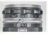
When taking infra-red pictures the distance setting obtained by facusing on the screen has to be adjusted before shooting. This is done by rotating the lens slightly, until the focused point on the distance scale is changed to align with a small dot on the depth of field scale.
