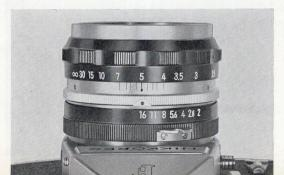
an F: 16 opening (F: 16 is shown in blue), the depth of field indicated by the blue colored lines on either side of the black indicator line will be between 7 ft. or 2 meters and 4 ft. or 1.2 meter approximately. This means that a picture taken at F: 16 with the lens focused at 5 ft. or 1.5 meter will show a range of acceptable sharpness between 7 ft. or 2 meters and 4 ft. or 1.2 meters.
