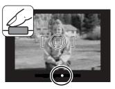
4. When the focus signal appears in the viewfinder, press the shutter-release button all the way down to take the picture.
