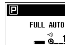
Example 2: Exposure-mode dial set to P , full-auto mode. Top part of display has turned black.
