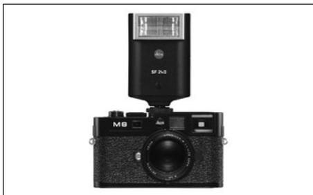
When attaching a flash unit to the LEICA M8.2 flash shoe (1.21), you should ensure that the foot of the flash unit is fully inserted and the clamping nut (if fitted) is tightened to prevent it accidentally falling out. This is particularly important for flash units with additional control and signal contacts, because if the flash shoe moves from its position in the flash shoe the necessary contacts can be broken, leading to malfunctions.
