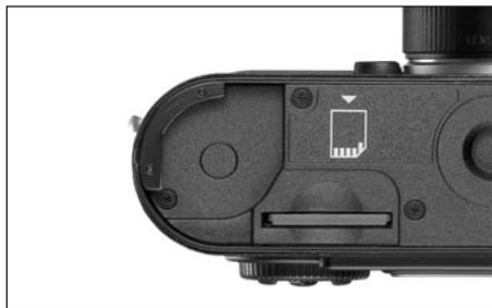
3. Insert the memory card into the slot (1.40) with the contacts at the back and with the beveled corner pointing downwards. Slide it completely into the slot against the spring resistance until you hear it click into place.
