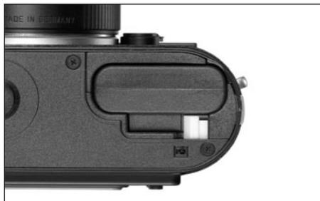
3. Insert the battery into the compartment with its contacts facing forwards. Press it into the compartment (1.38) until the white sprung locking catch (1.39) moves over the battery to hold it in place.
