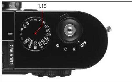
The size and position of the shutter speed dial (1.18) on the LEICA M8.2 are ergonomically optimized: On the one hand – even with the camera to the eye – it is very easy to use. On the other hand it is well protected against unintentional setting.
