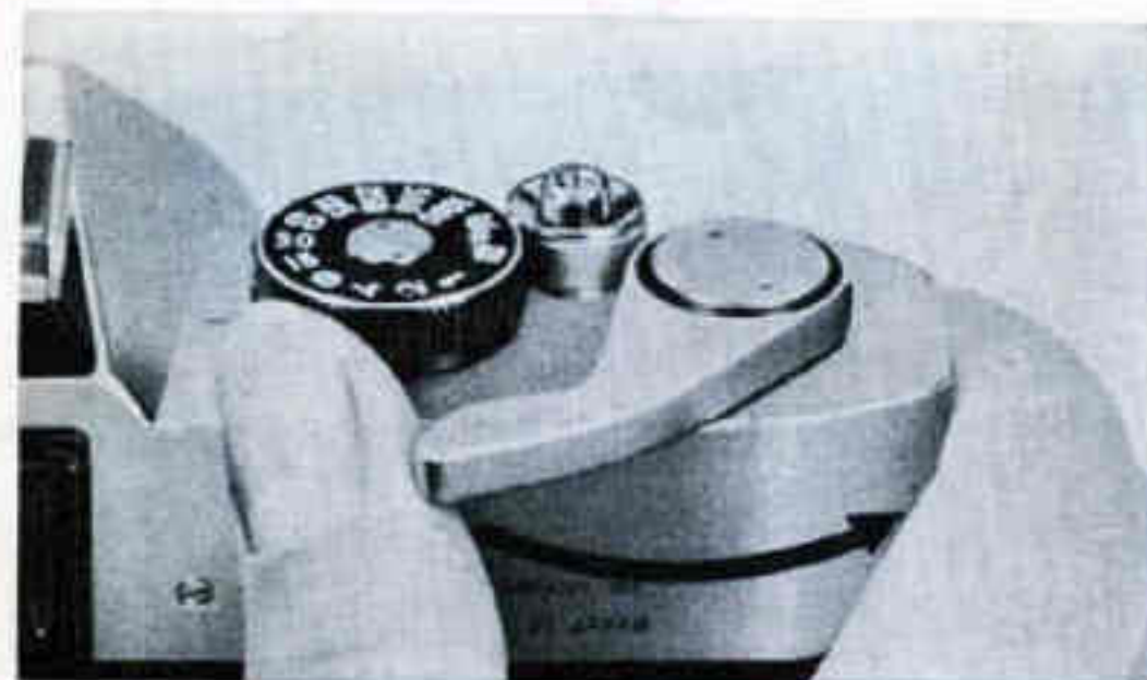
3. Wind the film advance lever.
