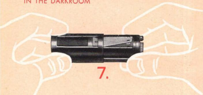
7. Slide the outer shell on to the inner with the mouth coincident. Draw out two or three inches of film.
