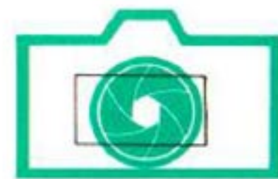
The shutter clicks. The diaphragm closes down to preset f/stop.
