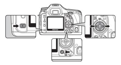
Press the ▶ button and use the four-way controller (◀▶) to select an image to be displayed first.
