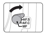
Look through the viewfinder, press the shutter release button halfway and turn the focusing ring.
