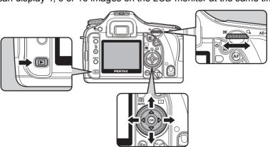
The default setting is 9-image display. The number of images can be changed but 9-image display is explained here.
