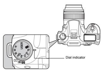
You can switch the Exposure mode by setting the icons on the mode dial to the dial indicator.
