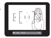
Use the four-way controller (▲ ▼ ◀ ▶) to select the desired AF point.
