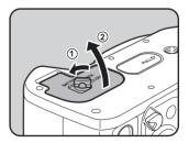
Face the A mark on the battery towards the LCD monitor, push the battery lock lever in the direction of the arrow (1) and insert the battery.
