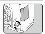
Insert the card all the way with the SD Memory Card label toward the LCD monitor.
