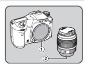
Align the red dots on the camera and the lens, and secure by turning the lens clockwise until it clicks.
