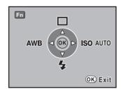
Press the four-way controller (▲ ▼ ◀ ▶) to set the operation.
