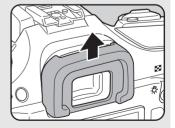
• If it is difficult to see the viewfinder image clearly even if you set the diopter adjustment lever, use the diopter correction lens adapter M. However, the eyecup must be removed to use this adapter. (p.216)
