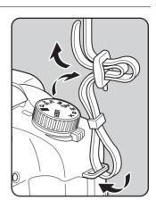
Pass the other end of the strap through the other strap lug on the camera, then secure it on the inside of the clasp.
