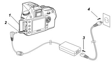
We recommend using the AC adapter kit K-AC10 (optional) when using the LCD monitor for a long time or when connecting to your PC.
