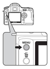
2 Use the four-way controller (()) to select the [Xi Set-up] menu.
