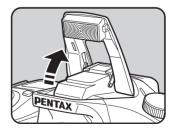
Switch between Auto discharge mode and Manual discharge mode (Flash ON) by pressing the **4UP** button while the built-in flash is popped up. If Auto discharge is set, appears on the LCD panel.
