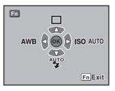
Press the four-way controller (O O) to set the operation.
